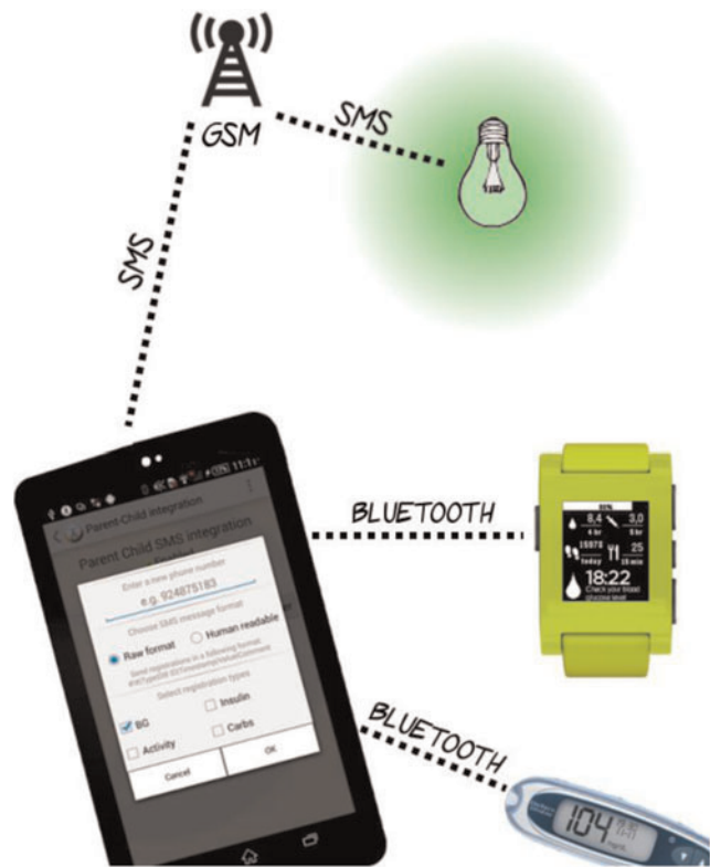
FIGURE 1. Available options for set-up of a new receiver’s phone number in the Diabetes Diary application and basic schema of data flow when authorizing the change of the light bulb’s color.
